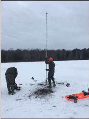
Sampling with the macaulay probe through a hole in the ice.
